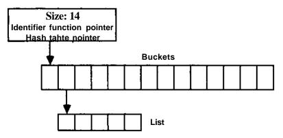
Figure 3-2: Representation of a Hash Table
